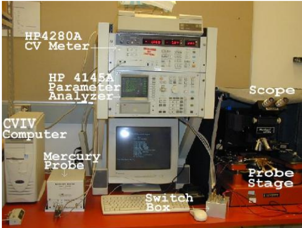
Photo 3: The main components of the CVIV system are labeled.
