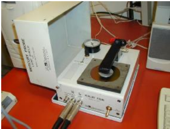
Photo 2: Closer view of the Mercury probe with the lid open.
