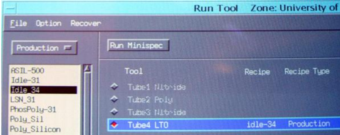
Fig. 4. The recipe and tube has been selected and the next thing is to select “Run Minispec”.
