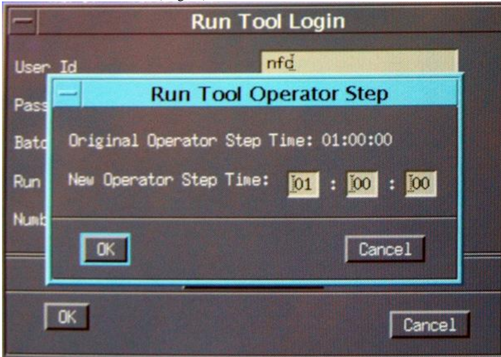
Fig. 6. The operator step, which is the delay time will determine the resulting film thickness.
