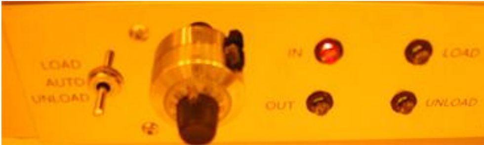
Fig. 9 The boat loader is closed, as the IN LED is lit, things are working correctly.
