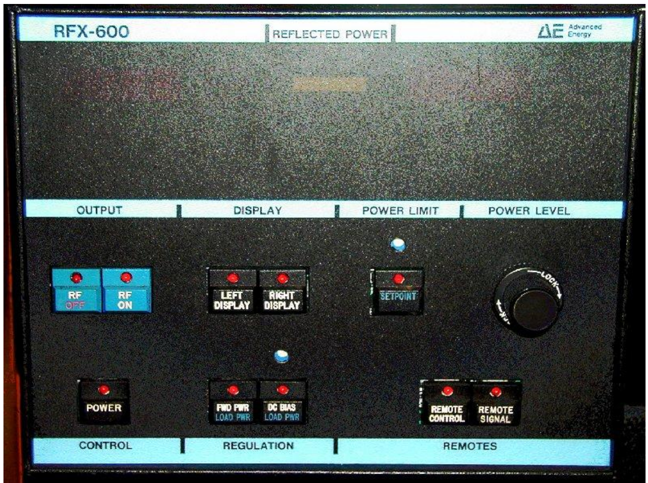
Fig 2. The ICP power supply control panel is used only when ICP etching is needed.
