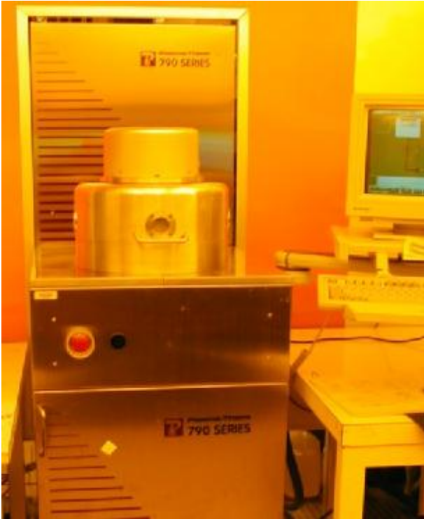
Fig 1. The PECVD system with the keyboard and monitor to the right of the system.
